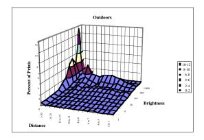
Figure 4. Photographic utilization space for a 35 mm nonsingle lens reflex camera under outdoor illumination conditions.
